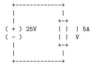
In the above circuit, a resistor is connected across a 25V voltage source and it is noted that 5A of current is flowing through the resistor. However, the resistance of the resistor is not given. We can once again solve for this missing variable using Ohm's law. By rearranging, we find that R = V/I, so R = 25/5 = 5 Ohm. Therefore, the resistor must be 5 Ohms in order to satisfy the given circuit.
