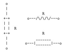
The blocky resistor model is typically referred to as IEC or "European" style, while the zig-zaggy model is referred to as US or "American" style.
