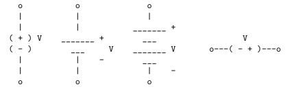
Voltage sources have (+) and (-) terminals, and a label beside them indicates the voltage across the two terminals. A 9V source, for instance, will satisfy the equation V+-V-=9, or there is a 9V difference between the voltage at the (+) terminal and the voltage at the (-) terminal.
